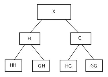
Nodes at each level of the wavelet packet tree can be *parent* nodes for *children* nodes at lower levels. An admissible wavelet packet tree has either 0 or 2 children nodes for each parent node.
