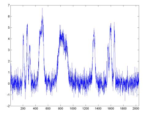
Denoise the signal down to level 3 using the Daubechies least asymmetric wavelet with 4 vanishing moments. Use the universal threshold selection rule of Donoho and Johnstone with soft thresholding based on the DWT coefficients at level 1. Use the periodization signal extension mode — dwtmode('per'). Plot the result along with the reference signal for comparision.
