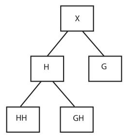
The wavelet packet transform can also operate on the output on the highpass filter. The following figure illustrates one *admissible* binary wavelet packet tree.
